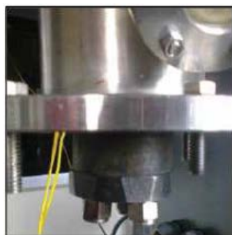
Figure 6: Bottom of the three catalytic beds in the lower flange of the reactor.
