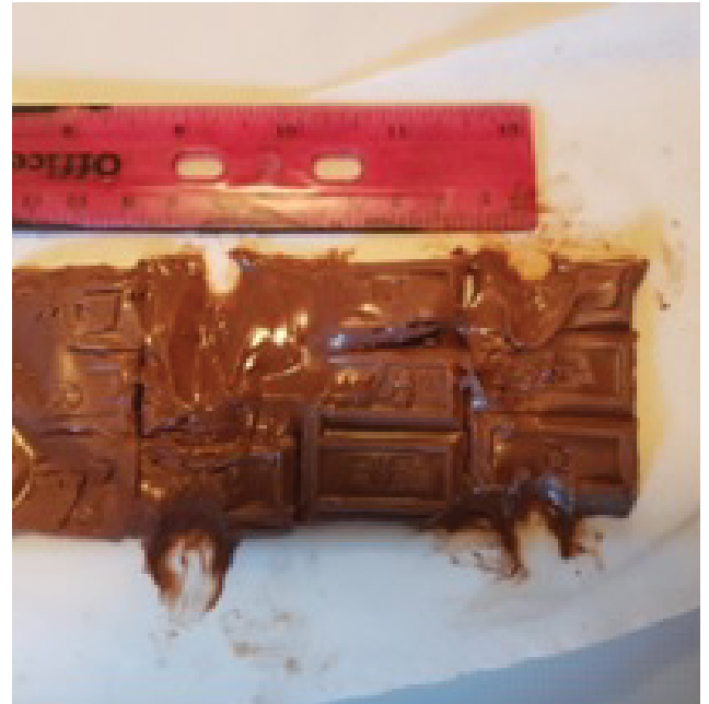
Figure 1: Melting bands (indicated by vertical lines) in chocolate substrate reveal the observed wavelength of microwave radiation. Vertical bands of melted chocolate are separated at an average distance of 2.65 cm in a microwave resonant cavity designed with a 2450 Hz magnetron. The resonant waves energize and induce vibration in molecules in the substrate which generates heat of melting. Temperature first rises at locations of EM radiation electric field maxima and minima. This separation distance is thus a half wavelength of the emitted radiation. The observed wavelength is twice this distance, at 0.127 m and may be used to estimate the intrinsic speed (but not the relative velocity) of the EM radiation.
