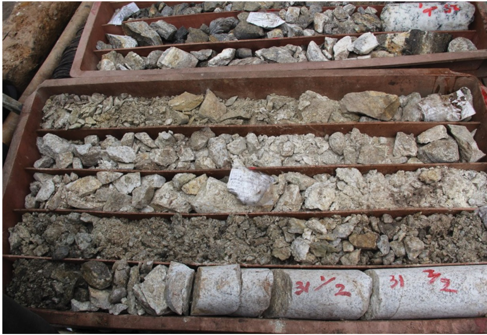
Figure 6: Rock cores showing that the deep cracked silicates underwent intensive carbonization. Large amounts of fine-grained yellow-brown secondary carbonates and clay minerals were therefore formed in the extremely deep silicate regions beneath the forest-wetlands. The secondary clay minerals held newly-formed organic matters normally.
